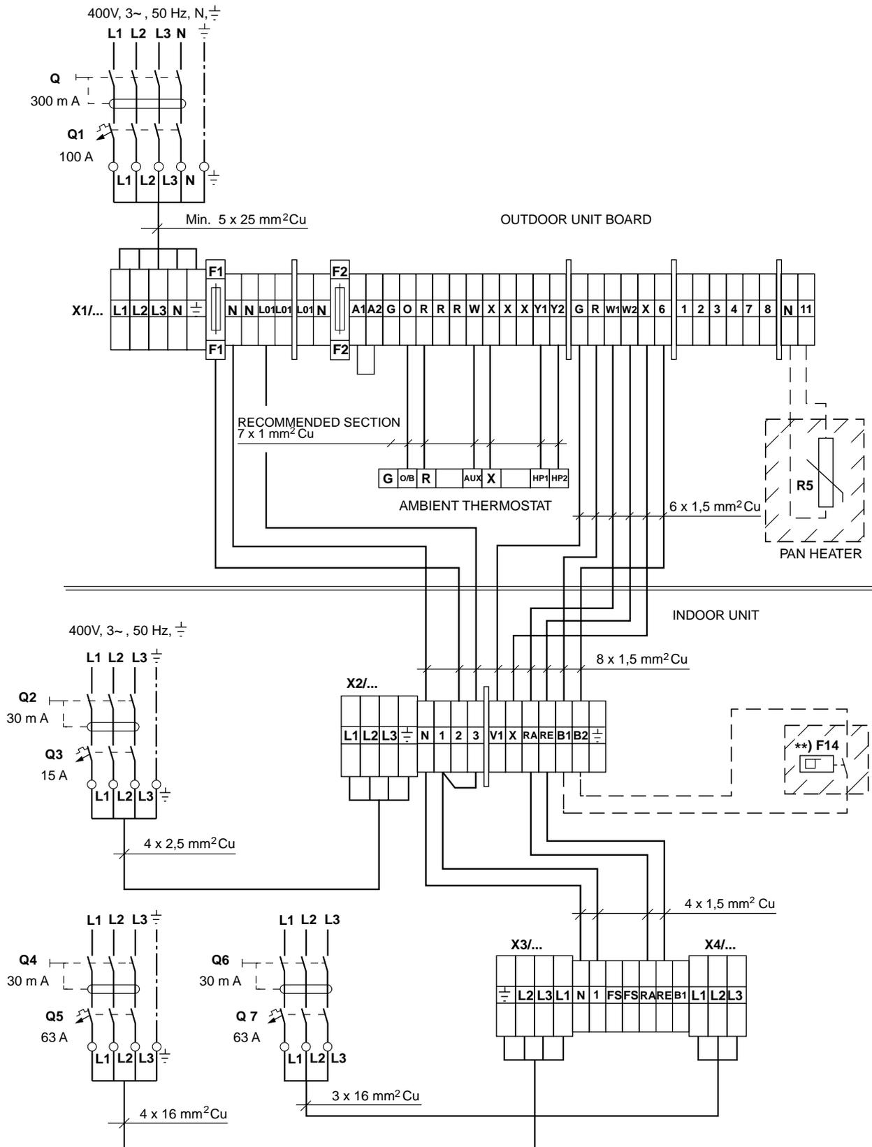
\*\*\*) WHEN AN ELECTRIC HEATER IS INSTALLED, FIT AN F14 AIR FLOW CONTROL
