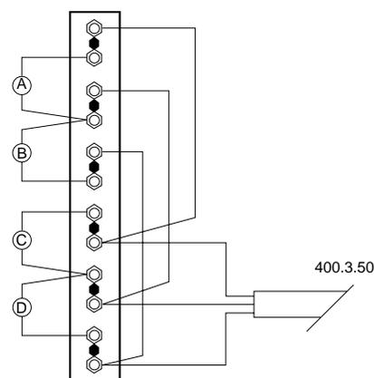
ELECTRIC HEATER CONNECTED TO 230V JOBSITE TRANSFORMATION
