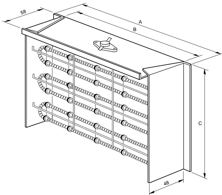
ELECTRIC HEATER CONNECTED TO 400V SUPPLIED FROM THE FACTORY
